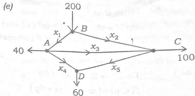
For the figure above find the general traffic pattern in the freeway network (Flow rates are cars/minute)
